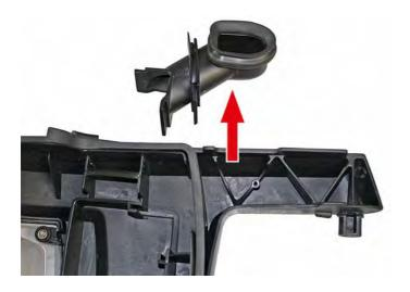
→ Remove the suction nozzle from the retainer towards the top.
