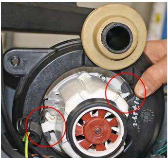
→ Mind the correct fitting position in the holder upon installation.
