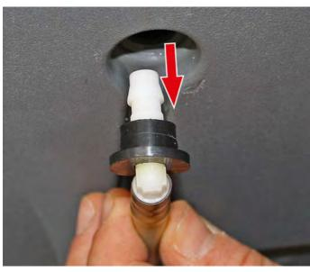
→ Pull the water level indicator out of the casing.
