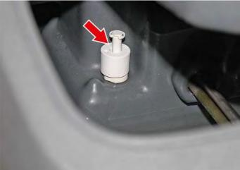
→ Remove the float switch from the fresh water tank towards the top.
